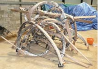
4m x 200mm x 25mm Oak is bent over the jigs and left to dry...
